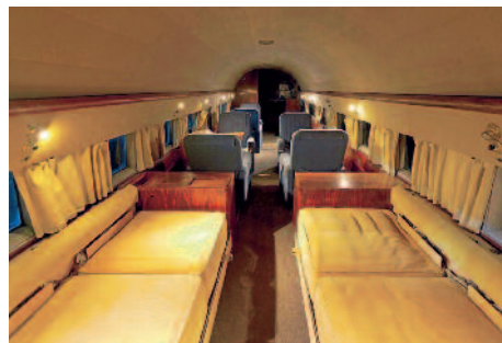
Grand Central Aircraft Manufacturing at Glendale fitted this luxury VIP interior with seating for 12. James Polivka
