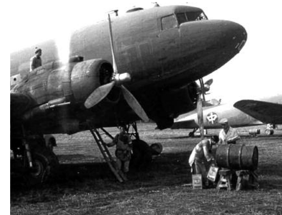
Conditions at some CNAC airfields were rudimentary. Captain Gifford Bull captured this image of C-47B Number 100 being refuelled by hand. Gifford Bull via CNAC.org
