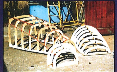
LEFT A spare engine side panel from Shuttleworth in place on K8203 to act as a pattern. BELOW The wooden formers for the new compound-curved cowlings.
